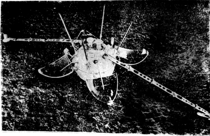
Unmanned Station "Luna-13" after Opening of Antenna Panels. At the Left: Extending Mechanism with Soil Probe-Penetrometer; At the Right: Radiation Densitometer with Transmitter.
